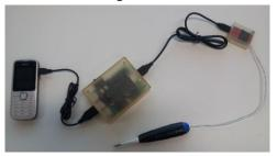
• Low-cost Fetal Monitoring Device based on phonocardiogram (PCG). Using cutting edge digital signal processing that separates and filters abdominal "noise" to detect fetal heart and body movement, pregnant mothers can be monitored and diagnosed for any maternal complications. Cheaper alternative to ultrasound, can be widely distributed to save lives.
